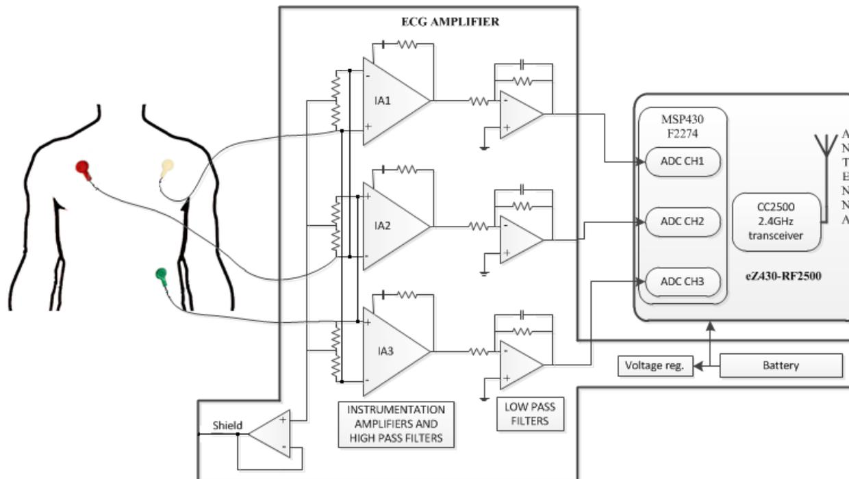
ECG amplifier connected to wireless module
