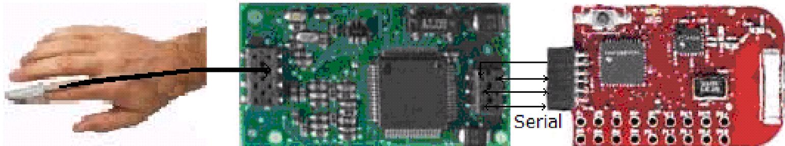
Micro Power Oximeter Board connected to eZ430RF2500
